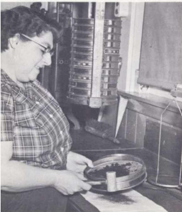
Below: Even the percentage of sand grains of a given size is important. Ida Flinton makes a sieve analysis of grain distribution of a molding sand
