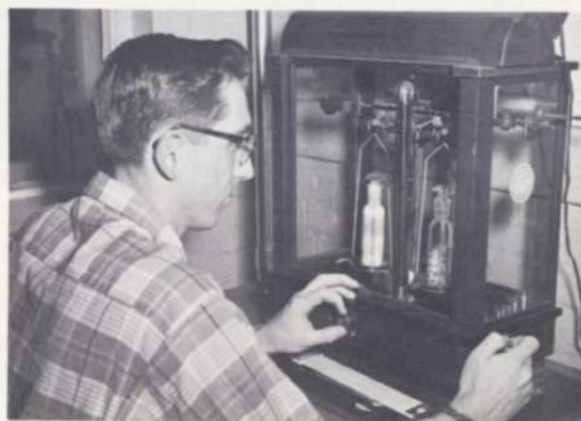
Scientific controls require exact measurements. Beginning a test, Donald Corkum weighs a sample on an analytical balance
