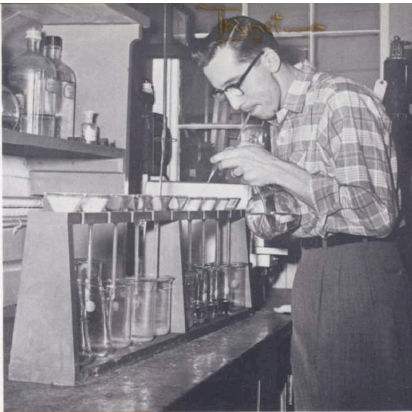
As part of a chemical analysis Donald Corkum filters a solution in a test of cast iron. When he has finished he will have determined the per cent of silicon present in our iron
