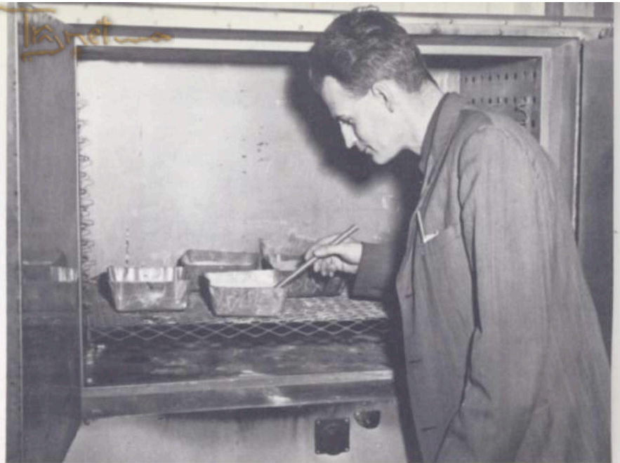
To our Foundry, the properties of sands and clays are of great importance. Assistant Metallurgist Gerald Markhard checks a clay sample being treated in an electric drying oven
