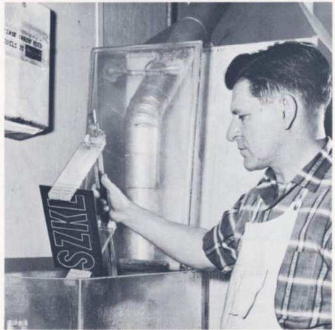
Drawn letters are photographed and etched into zinc plates which serve as the patterns for the engraving of the master matrix
