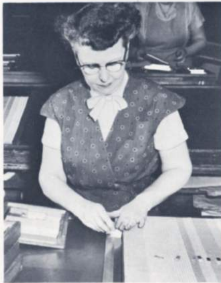
Rows of individually cast letters are assembled in complete fonts which have the required number of letters and symbols in the correct amounts for use in the English language according to frequency
