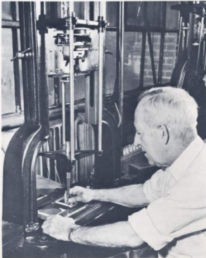
The Benton engraving machine is an ingenious device to engrave the letter in actual size upon a master matrix. By tracing the pattern plate this instrument reproduces and repropotions the character in the desired size
