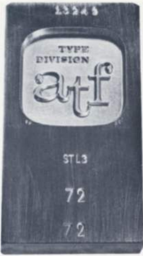
Pictured is a matrix from which the type next to it was cast. This type is known as logotype which is a single type body containing two or more letters
