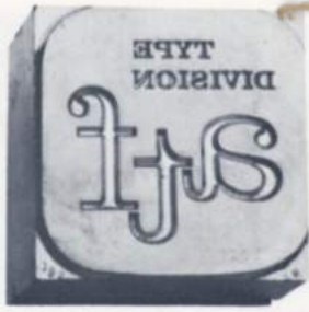
Pictured is a matrix from which the type next to it was cast. This type is known as logotype which is a single type body containing two or more letters
