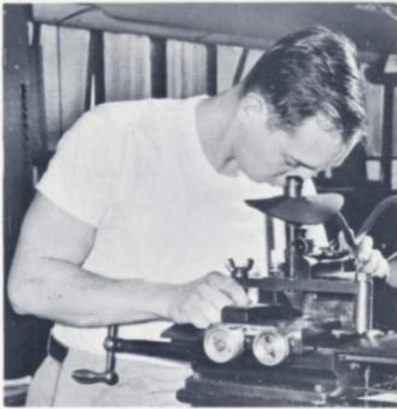
Here the finished matrix is trimmed and smoothed to exact size and the engraved letter image positioned accurately to combine well with all its neighbors
