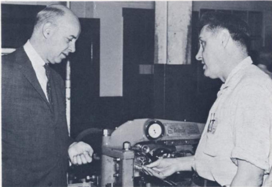
Mitchell Nadolink, Department 425, explains his idea of knurling to size all 5/16" Unitrol shafts to General Superintendent John H. Cunningham. Submitted as suggestion #58-187, Mike's idea eliminated a grinding operation and brought him an award of $105
