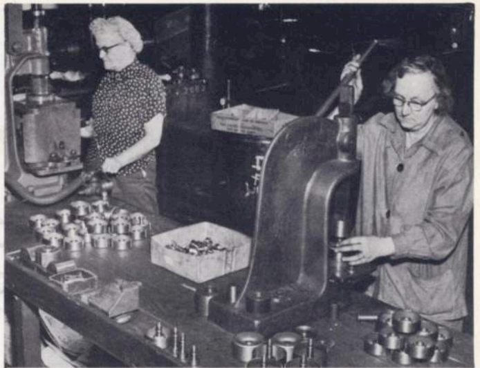
Above: As simple a part as a pulley requires several operations. On the right Mrs. Anna LeBlanc presses bearings into pulleys while Mrs. Rose Proulx, left, crimps bearings firmly onto the pulleys for spinning frames and twisters
