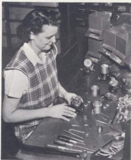
Above: Department 429, in addition to furnishing parts for the erecting floors, makes a number of complete assemblies. Here Mrs. Mabel Lemoine assembles a hank clock from the parts in the containers before her. Below: Francis Ledue is a specialist in the cutting and joining of chain. He is shown making up chain to the proper length for a builder motion on a spinning frame
