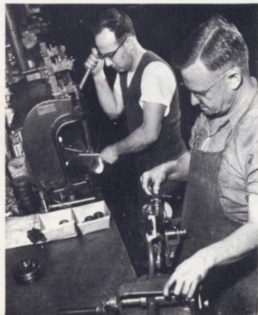
Below: Many other small parts must be sub-assembled. On the left Jacob Sohigian presses keys into shafts. On the right Edgar Baker assembles a cotton builder
