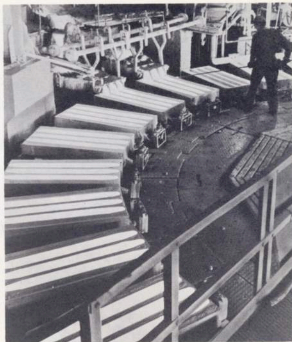
The copper cathodes are remelted and cast into shapes suitable for making sheets, pipe, or wire. These bars will be drawn into wire
