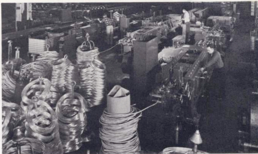
The copper cathodes are remelted and cast into shapes suitable for making sheets, pipe, or wire. These bars will be drawn into wire
