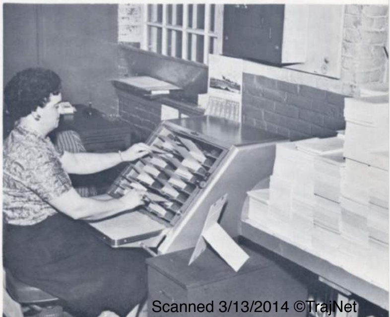
The plate is placed in one of three Whitin duplicators where Marcelle Lucier runs off the required number of copies. Speed range is from 3400 to 7200 reproductions an hour. An average of 30,000 copies can be made from one plate
