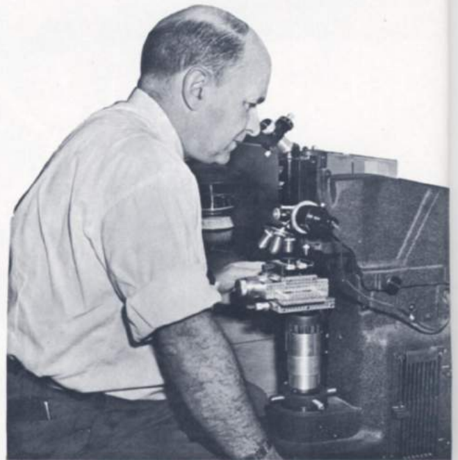
Above: Experimental Machining is concerned with such details as the hardness of cross sections in parts as small as a needle. The Tukon Tester being used by Arthur Jackman, metallurgical engineer, is so exact that fourteen separate readings can be made in the thickness of a razor blade
