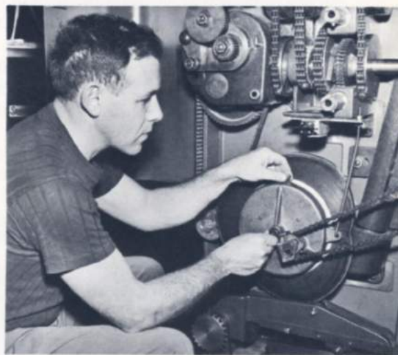
Kenneth Stanley adjusts the pick motion on a Piedmont Spinning Frame. Such maintenance of the exhibition machinery in the Research Division is one of the secondary functions of the department
