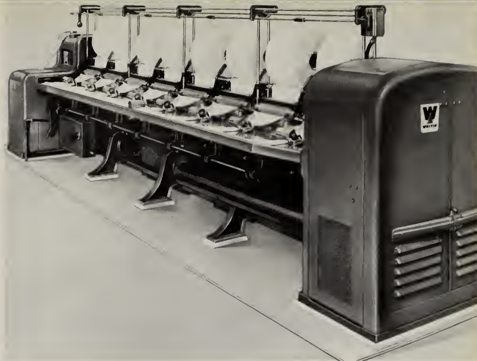
The laps, weighing 1,000 grains per yard, are the supply units for the Whitin J5 Comber, the world's most advanced Comber
