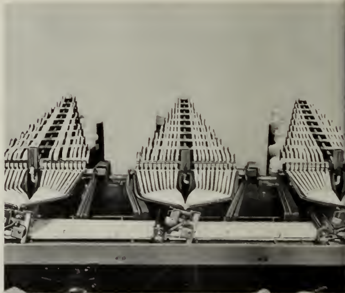
On the Super Lap up to sixty slivers from the M Drawing Frame are drafted and combined into a supply unit for the J5 Comber. The Super Lap produces up to 500 pounds per hour—enough laps to keep about eight Combers working
