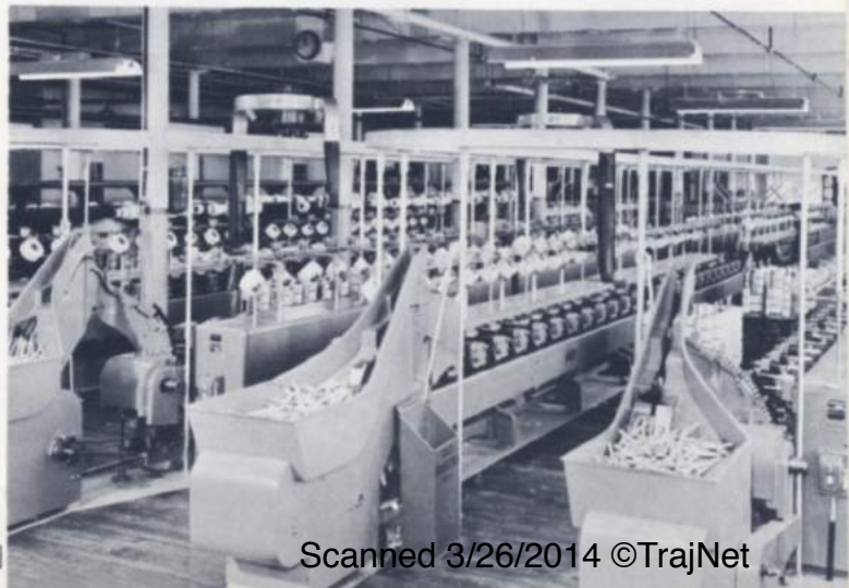
Mill installation 192 spindles Whitin Speed-Matic Winders with bobbin loaders
