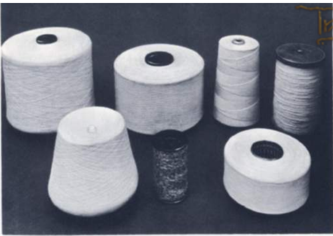
The purpose of a Filling Bobbin Winder is to take yarn from a variety of supply packages, such as those at the left, and rewind the yarn onto filling bobbins such as those shown at the right
