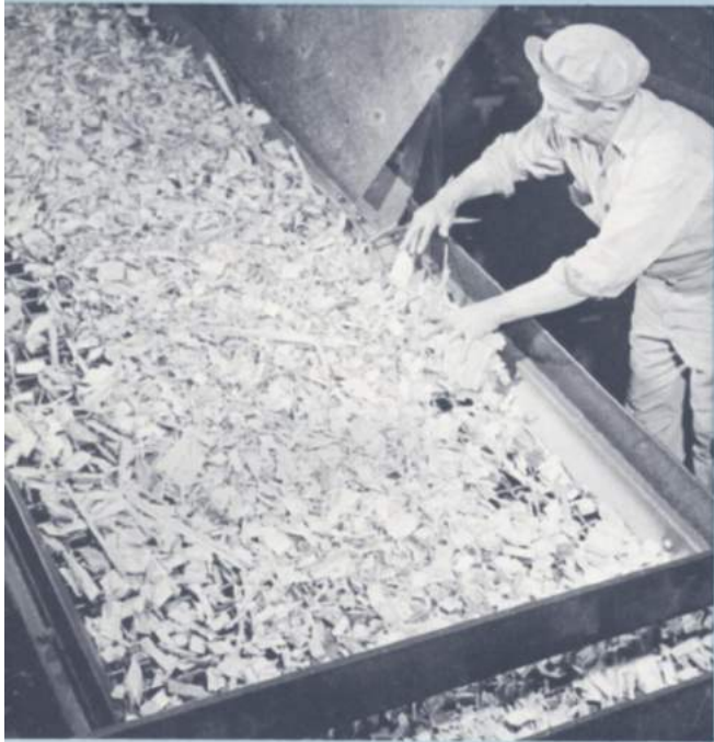
The logs, now free of bark, are reduced to chips by massive, high-speed equipment. Under the supervision of a workman, the resulting chips are screened of knots and sawdust as they are conveyed to storage bins
