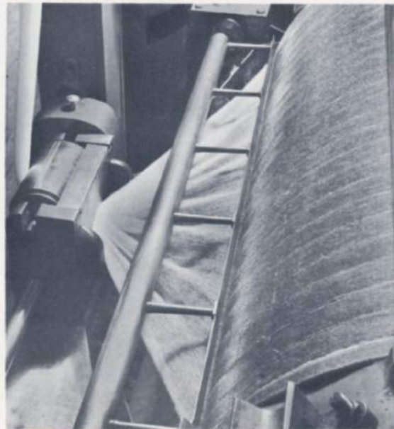
The cotton fibers come from the doffer in the form of an exceedingly fine web, separated from the doffer surface by the rapid up-and-down movement of the comb. It is condensed into sliver by being drawn through a trumpet by calender rolls. A uniform web with few neps is a sign of quality carding
