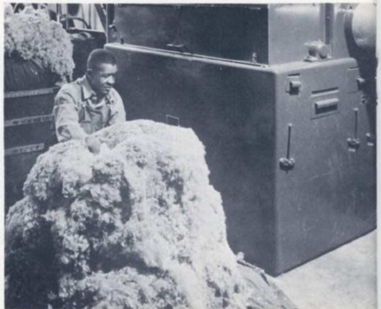
This is a mill photograph of the actual droppings in the cleanout chamber of an Axi-Flo, showing the type of trash which is removed from the usable fibers. The trash contains almost no usable fiber. The fibers shown are immature ones known as notes
