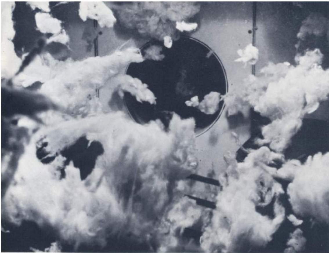
This high-speed photograph of the interior of an Axi-Flo shows tufts of cotton in the process of being opened and cleaned
