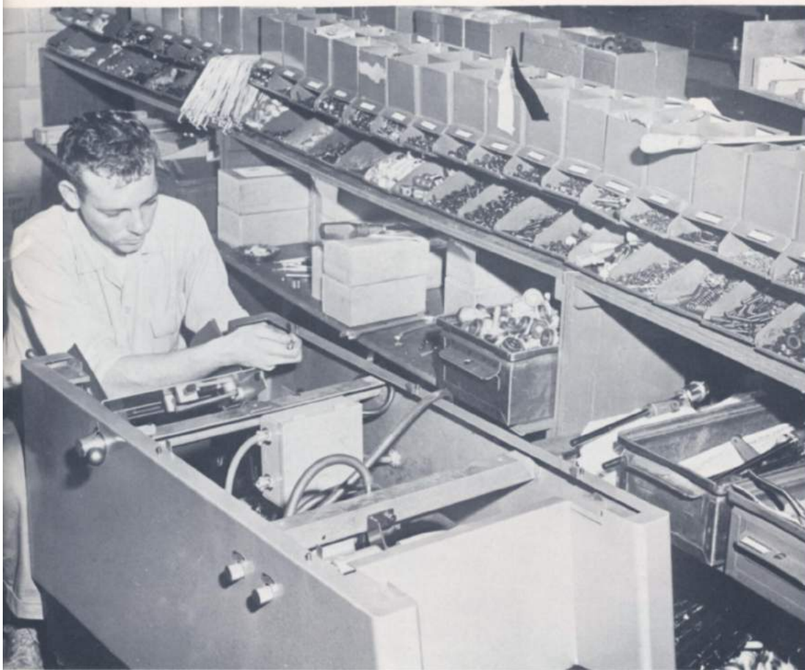
As each of the components passes down the assembly lines, parts are added to it from conveniently arranged bins. This reduces the amount of time needed to secure a needed part and speeds production. Here Normand Bussiere attaches a collecting tray to a base
