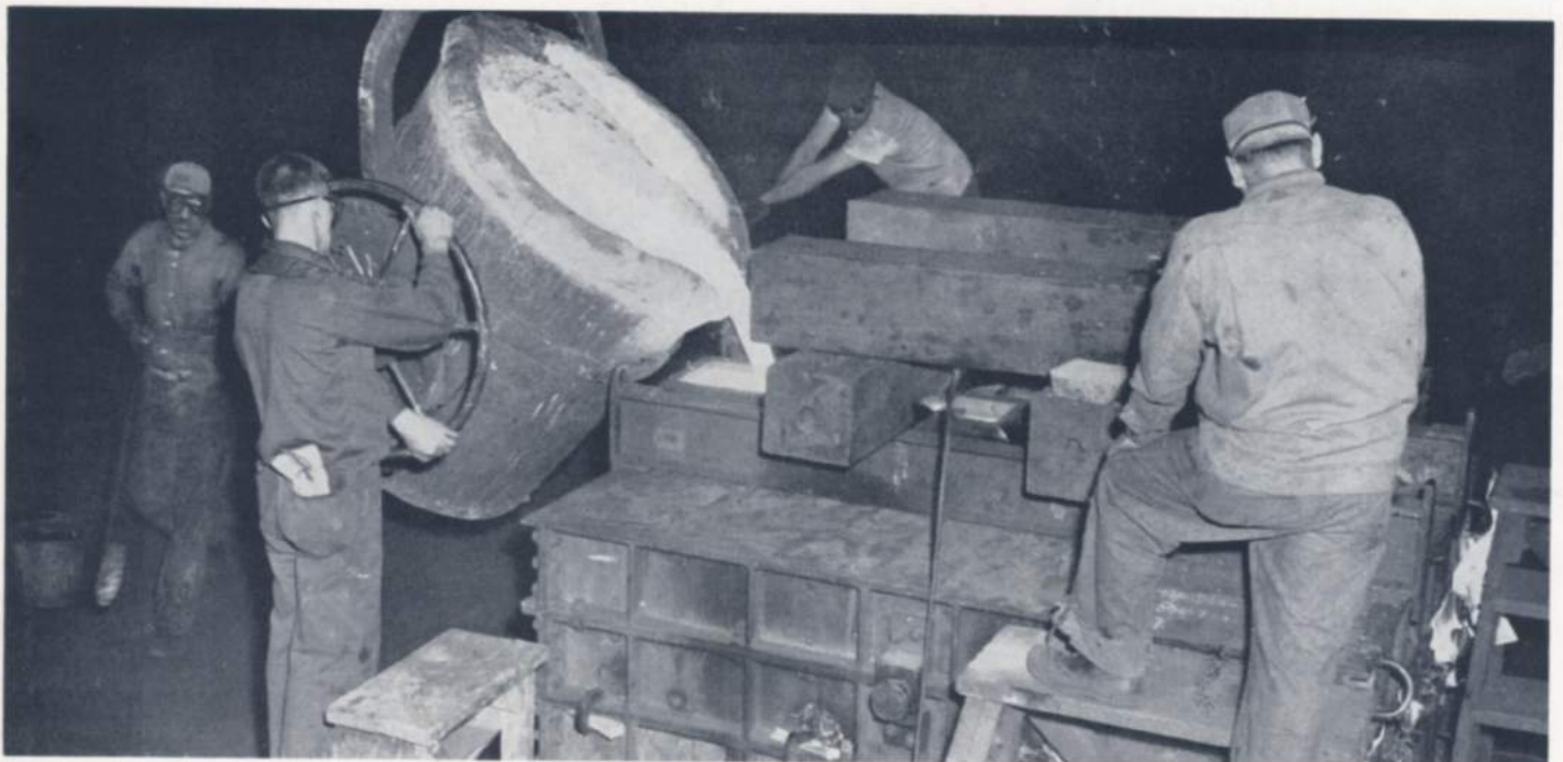
In a matter of seconds 6,000 pounds of molten metal are poured into the mold. From the left: Ernest Julien, Robert Hoisington, Allan Jenkins, and Alfred Marchand
