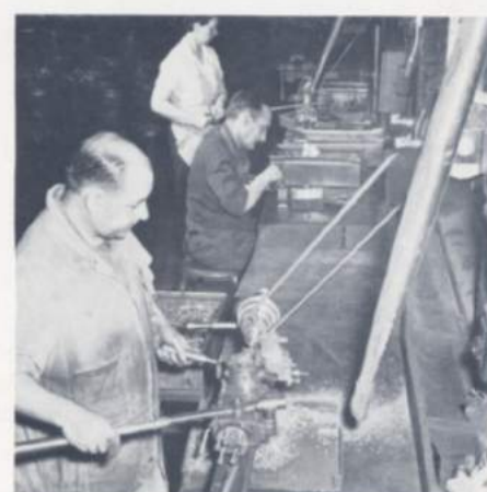
George Sesona and Margaret Fallon machine bolster steps on turret lathes while Rouville Lalanne, center, assembles oil caps on bolster cases
