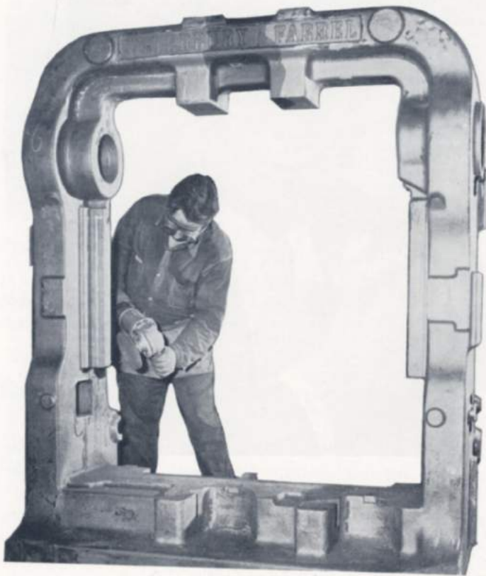
Franklin Maynard, Department 405, is shown snagging a mighty main frame casting for a Waterbury Farrel bullet press. Two cranes and a lift truck are needed to place this casting in the Roto-Blast
