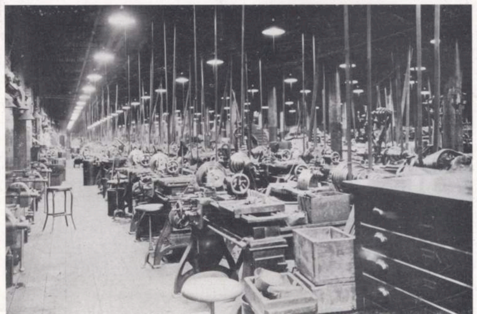
Spinning Job. Notice the Absence of Shadows Under the Stools or Elsewhere. A Sign of the Best Lighting
