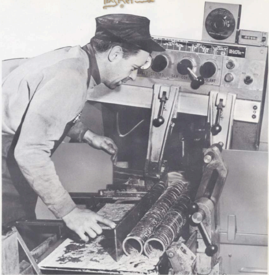
Steel rings are no longer made from forgings at Whitin. All rings are now cut from steel tubing. After the saw-cutting operation in the Steel Cut-Off Department, the blanks are sent to the Ring Job for machining. Damase Garipey is operating the saw-cutting machine
