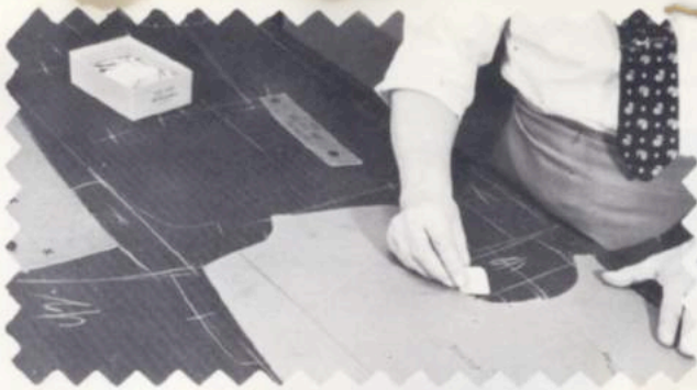
Chalking the pattern. Patternlayers take particular care with stripes, plaids and checks to insure a perfect continuity in the pattern where seams join and pockets overlap. The cutter must follow the chalk line so accurately that he literally splits the line as he cuts
