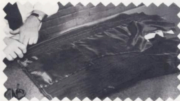
Lining basting is carefully done by hand and distributes fullness so that the coat will hang evenly and the lining itself will not bind or constrict
