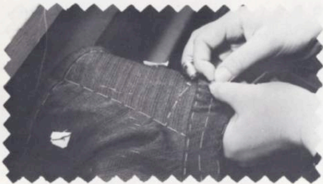
Collar basting joins the top collar to the coat, following the contours of the undercollar; gorge basting joins the collar to the lapels. The collar points are carefully shaped and care is taken to align the fabric pattern with that of the coat
