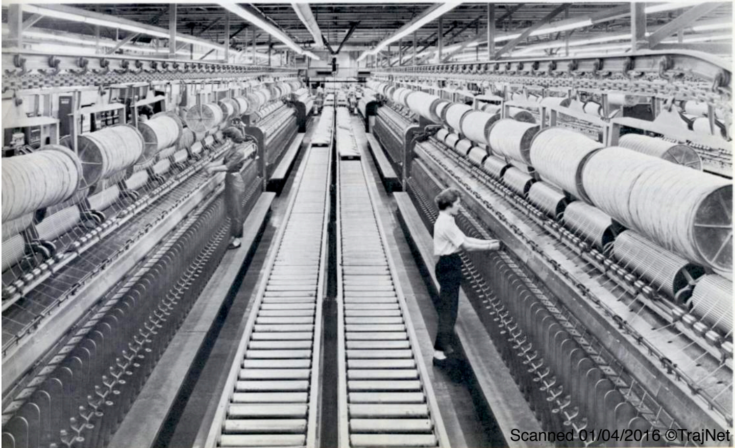
Alley view of Wool Spinning frames showing modern conveying methods. Spools are handled on overhead carriers while filled bobbins are transported on roller tables to twisters in background
