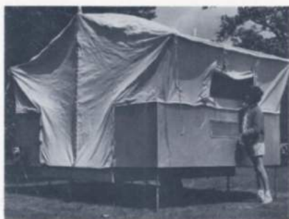
The top of the trailer consists of heavy-duty canvas with front and rear screened doors and two screened windows. In open position, the canvas is stretched over a ridgepole and locked in place
