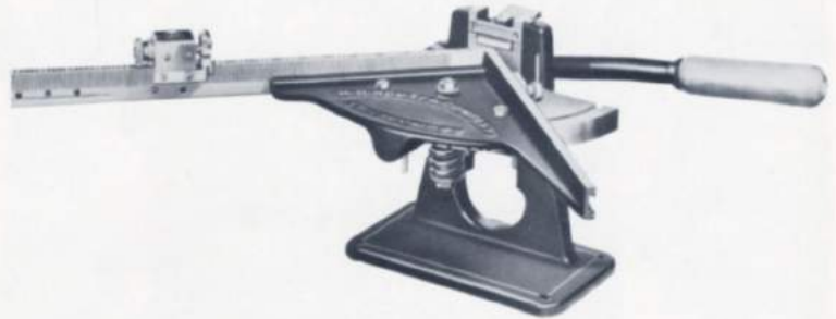
A Nelson saw used to cut type and plates
