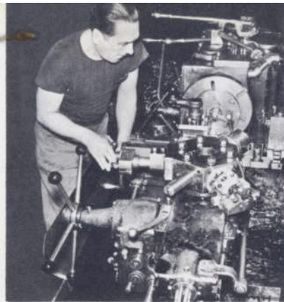
Lionel Grondines uses a Warner Swazey turret lathe to cut threads on a winder part
