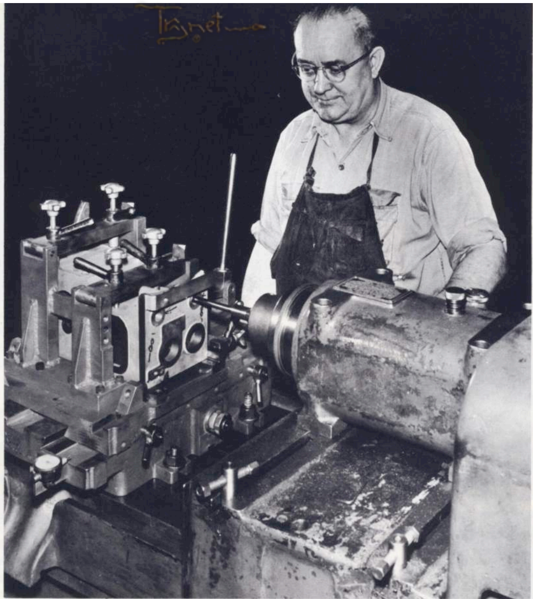
One of the most useful machines in Department 423 is the Heald Borematic. Arthur Ashworth bores an oscillating shaft hole in a winder box
