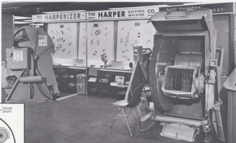
Front and side view of 18" Harperizer. This machine can smooth as many as 600 small parts at one time. Removable dividers in 37" long barrels form compartments which make it possible to process parts of different sizes
