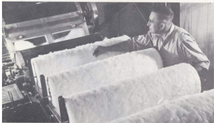
Left: Finisher picker continues fiber blending and forms a uniform lap for processing on the card. Four or more laps are doubled on this machine
