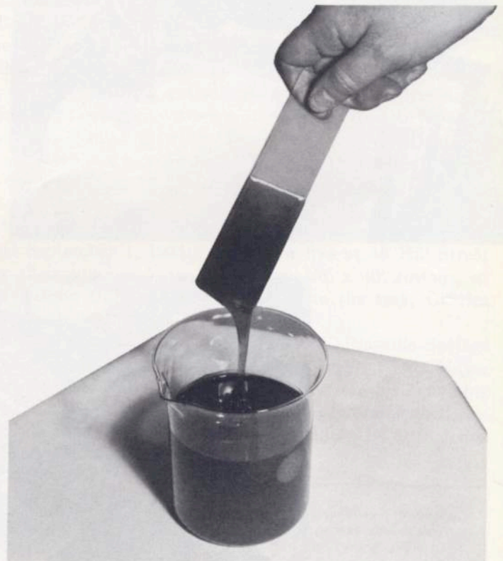
The cellulose xanthate crumb is now mixed in a weak solution of caustic soda in a machine where revolving blades beat and mix the substance. In this step, the cellulose xanthate crumb is converted into a liquid known as "viscose solution"
