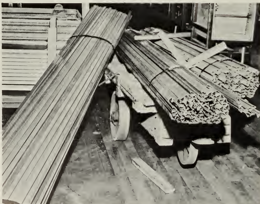
Luckily no one was injured when this large bundle of creel channels rolled off a four poster platform truck. This is a case where the stock was just too heavy for the steel rods supporting the load. Many of the channels were badly damaged and could not be used in their original lengths. Very careful attention is required in loading operations
