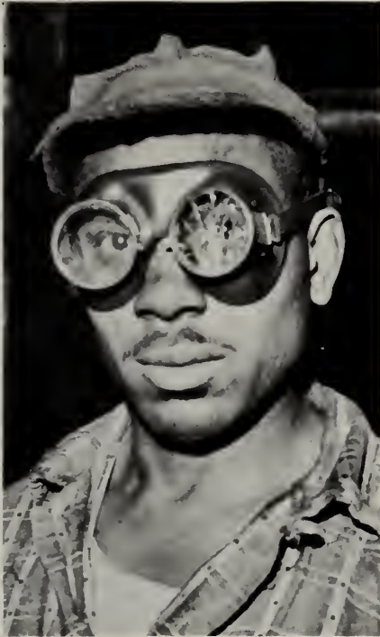
Maurice Chapman, Cast Iron Room, is another man who knows the value of wearing safety goggles in a hazardous area. A chip flew from an abrasive wheel, which he was dressing, and struck the center of the left lens as shown
