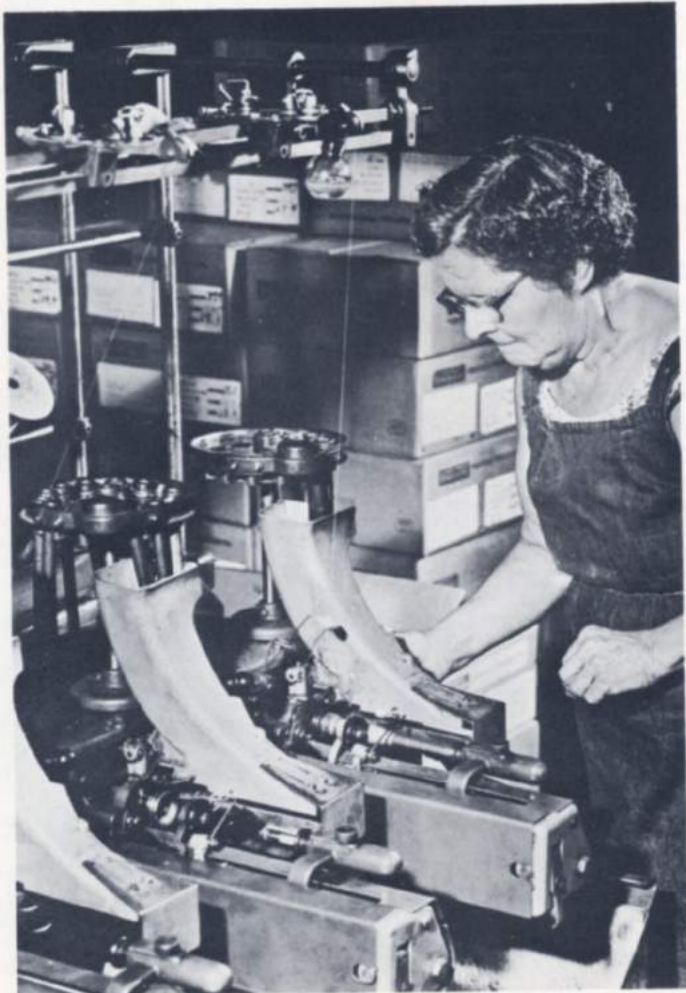
Whitin-Schweiter Winders are used in winding six hundred feet of Fiberglas yarn onto quills at U. S. Steel's Cyclone Fence plant at Greensburg, Indiana. The quills hold the wool or horizontal threads in the loom
