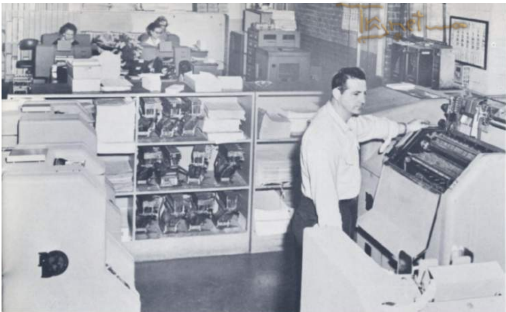
A.T.F. Customer Records Department, where a Remington Rand Univac is used to record all transactions with customers and all basic data on each account
