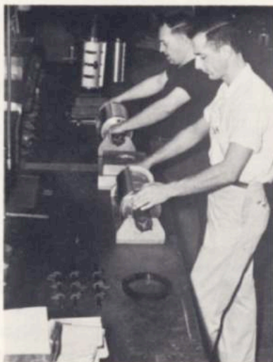
MODERN TECHNIQUES of cold-forming metal speed production. Here Gordon Thomson, a set-up man, adjusts a thread-rolling machine for operator Dorica Thompson who is threading duplicator cylinder shafts
