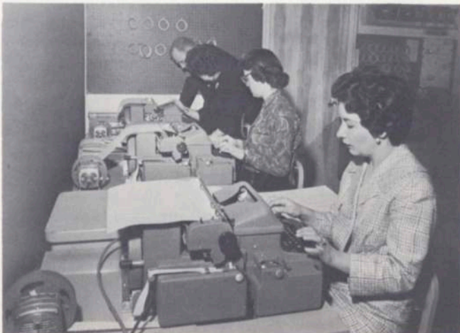
Operators simultaneously produce control tape and hard-copy "proof" on ATF Typesetter Keyboard Units at Tweddle Litho. High-speed phototypesetting battery has been added as part of Tweddle Litho's expansion program, enables fast-growing Midwest plant to offer buyers a complete one-source offset printing service, from rough copy to finished product
