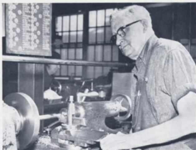
Conrad Watier turns a stud for another small repair order
