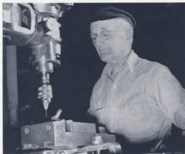
Below: William Boudreau, who has been here since March, 1926, drills an air hole in a boring tool
