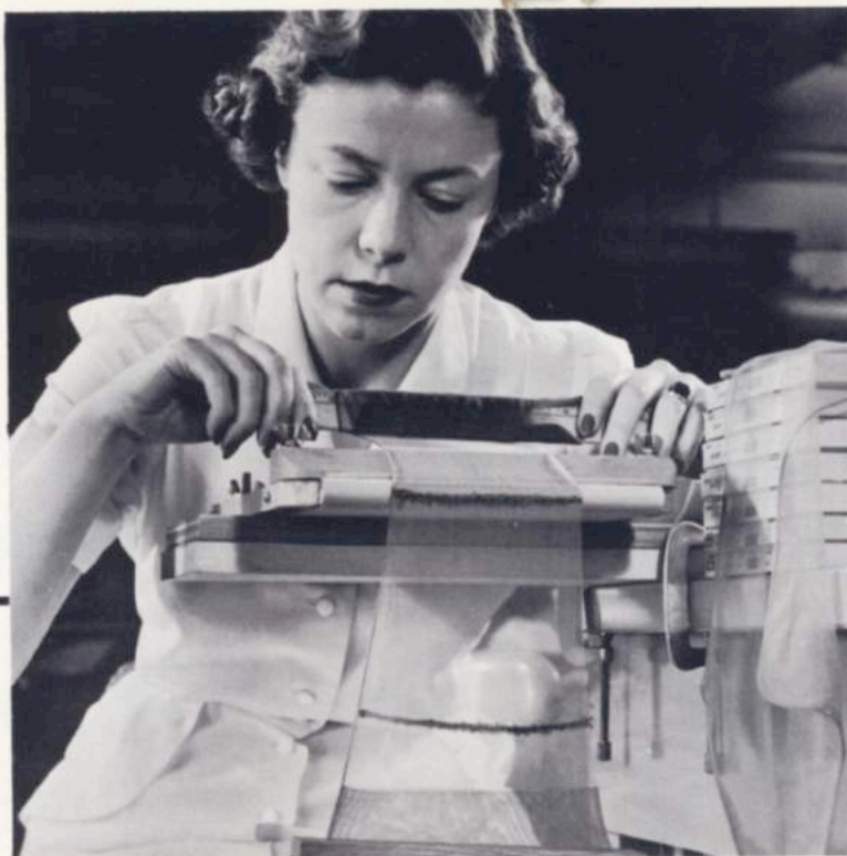
SNAGGING WOMEN'S HOSE—ON PURPOSE! Women's sheer hose of good quality must be snag-resistant. This technician is subjecting the hose to the action of sandpaper and counting the number of snags produced
