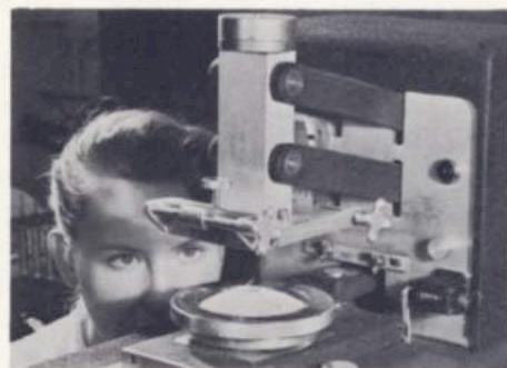
HOW MUCH WEAR WILL A MAN'S SUIT TAKE? Will this fabric make durable suits for men? This device gives the answer. A specimen of suiting is stretched taut over an inflated rubber diaphragm and subjected to the rubbing action of specially selected abrasive paper. This test simulates the abrasive wear that occurs on trouser seats and the back of trouser legs. Fabrics must withstand several hundred cycles of this accelerated wear test to get a satisfactory rating
