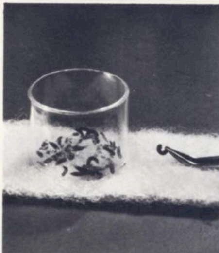
BLANKET SAMPLES TESTED FOR MOTH-RESISTANCE. Closeup view of black carpet beetle larvae used to test moth-resistance of blanket sample. Possible damage by moths and black carpet beetles is countered by chemically treating blankets during manufacture
