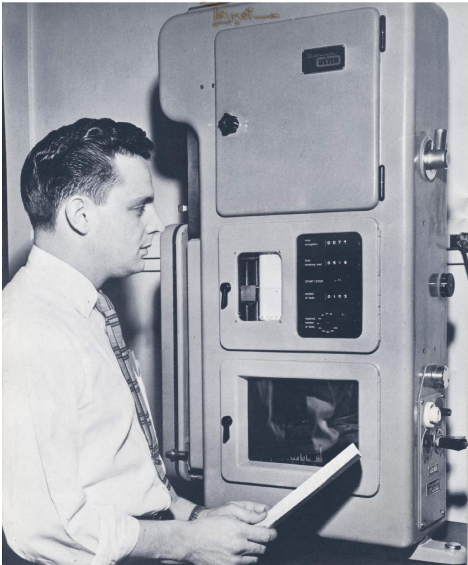
Visitors to the laboratory are often fascinated by the Uster Single Strand Tester here being used by Hugo Meotti, laboratory supervisor. This machine may be set to break from twenty to two hundred samples from a bobbin of yarn. Electronic, it not only records the elongation and breaking strength of the yarn but also forms a frequency chart by dropping tiny balls into slots. In some ways it resembles a pinball machine
