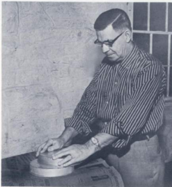
At the time the pictures were taken, Ralph had completed the grinding of his mirror. Using two tin pans which in size and shape resemble the blanks from which the mirrors are ground, he demonstrates the method by which the mirror is ground to the proper focal length
