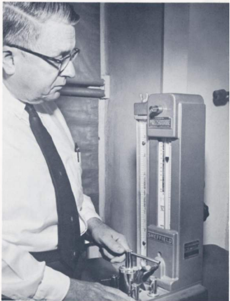
The quality of a yarn starts with the quality of the fibers from which it is spun. Arthur Adams, who has charge of the Demonstration Floor, uses a micronaire to test by compressed air the fineness of individual cotton fibers
