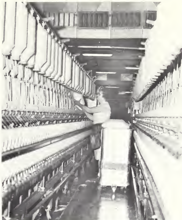
New spinning frame creels to accommodate the large raving packages are too high for creel roving to be placed on top of the creel. Spinners creel from the raving frame doff boxes. Only 37% as much creeling is done now as formerly
