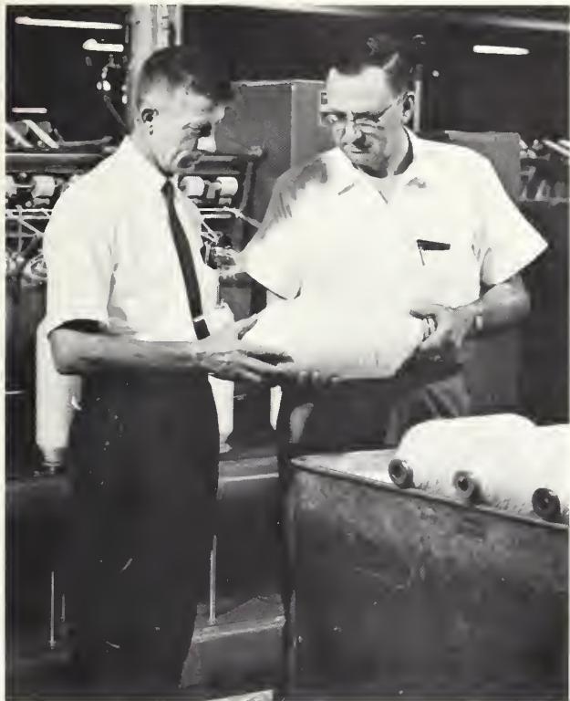
Dan Melton, Superintendent, left, and Lester Stearns, Foreman, examine the 78-oz. 14" x 6½" bobbin of roving produced by the "Scotsman." New Spinning frame creel boxes, three to a roving frame doff, are used in doffing the frames
